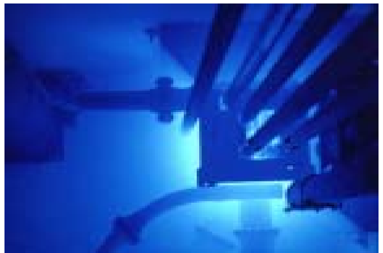
The OSU Research Reactor seen through the reactor pool from above. The blue glow is Cherenkov radiation, which is visible light emitted when charged particles are travelling through a transparent substance (such as water) faster than light travels through that substance. For more information: http://www-nrl.eng.ohio-state.edu/
