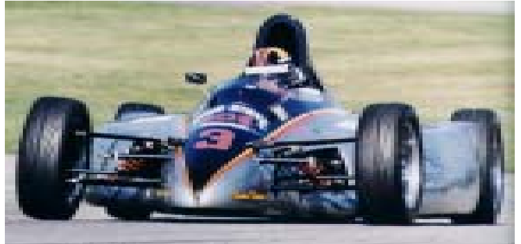
The Smokin' Buckeye is an electric car built by the Society of Automotive Engineers (SAE) Formula Lightning Team. The 2001 version maxed out at 144.2 mph. It runs on 31 12-volt Optima lead acid batteries. http://www.smokinbuckeye.com/
